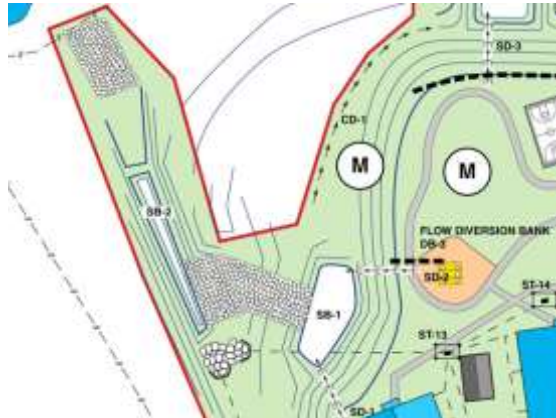
Sediment basins SB-1 and SB-2 in series
