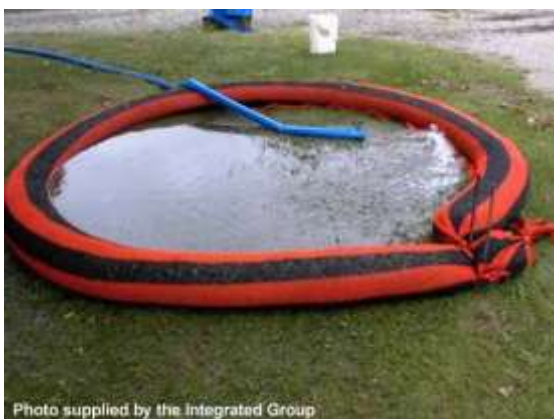
Compost-filled filter sock
