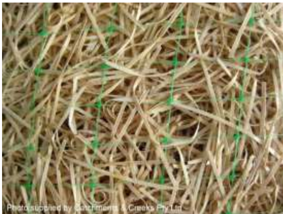
Temporary erosion control mat
