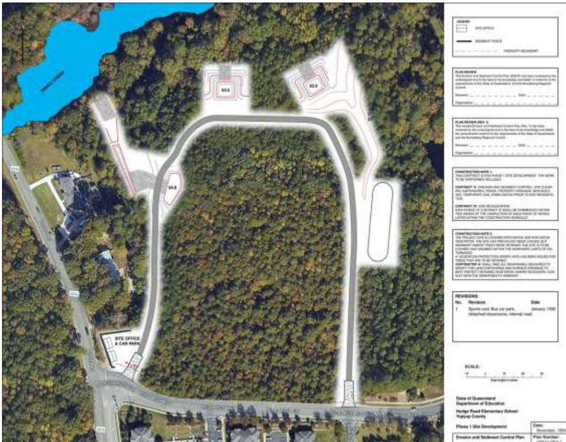
Figure 16 – Initial land clearing to allow construction of the sediment basins
