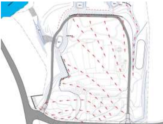
Post-earthworks drainage plan
