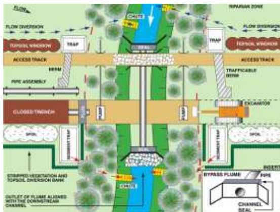
Cofferdams with gravity bypass
