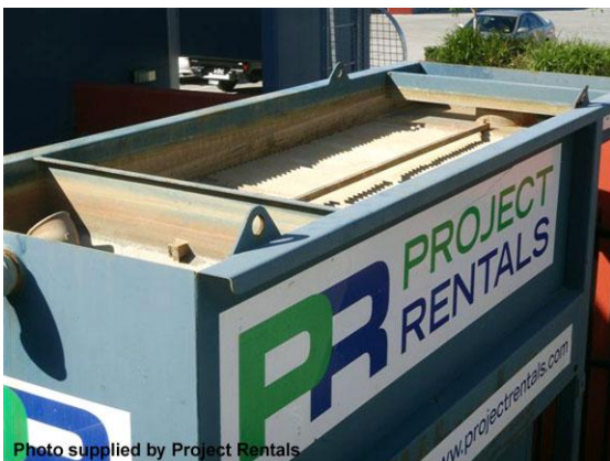
Lamella settling tank
