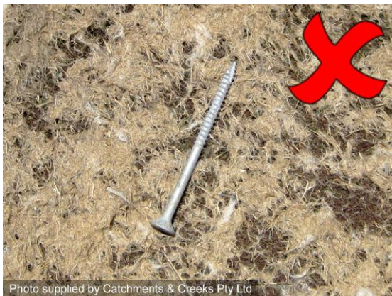
Wood screws used to anchor a blanket
