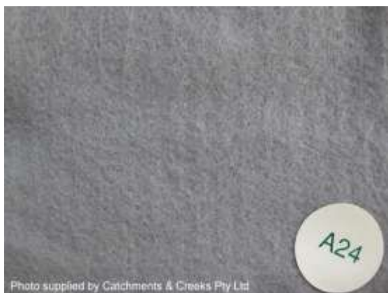
Filter cloth underlay
