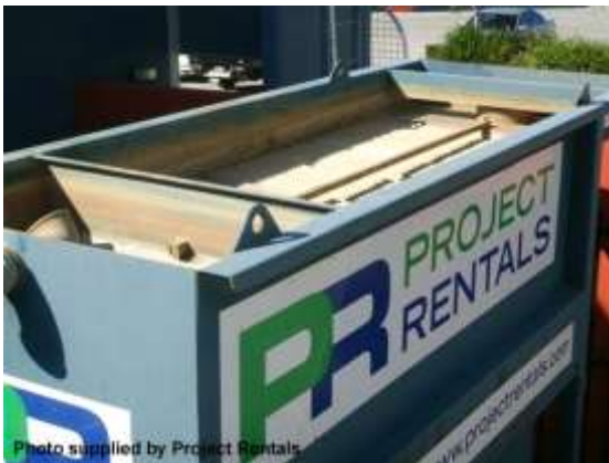
Lamella settling tank
