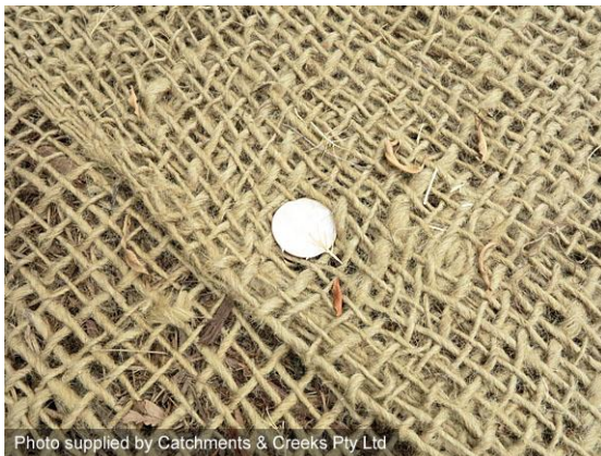
Erosion control mesh
