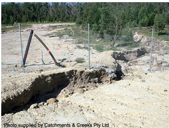
Gully erosion in slaking soil
