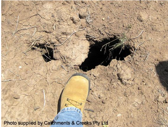
Tunnel erosion above pipeline
