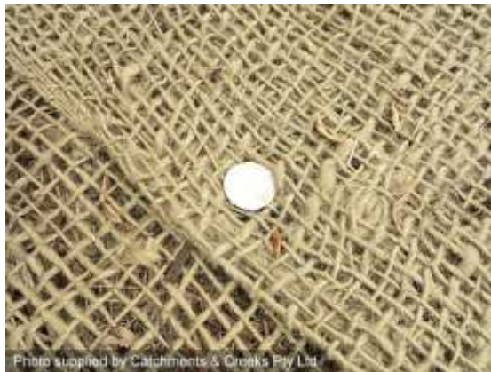
Erosion control mesh
