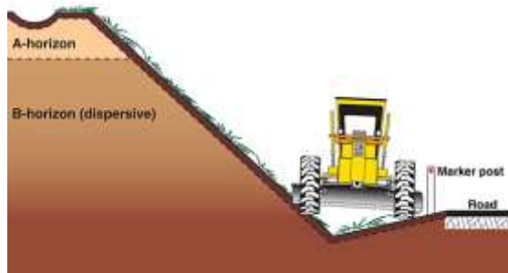
Mechanical disturbance of batter toe
