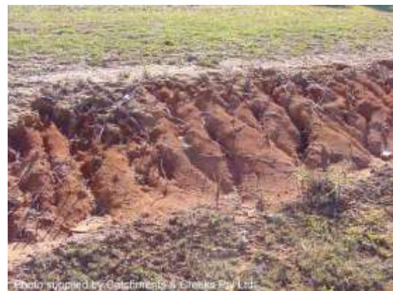
Fluting of the exposed dispersive soil
