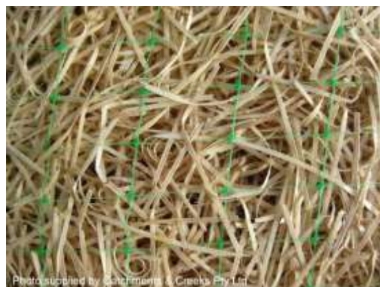
Non UV-stabilised synthetic composite mat
