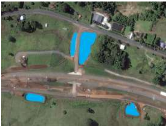
Sediment basins on road construction
