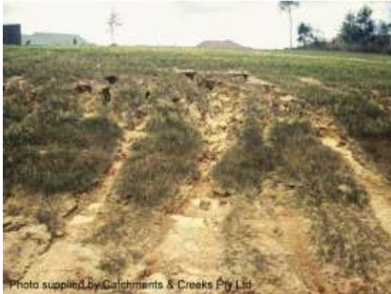
Directly seeded dispersive soil
