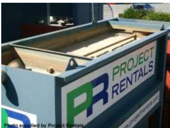
Lamella settling tank
