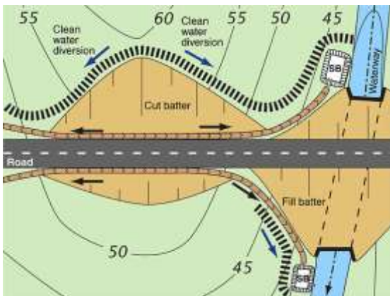
Drains directing water to sediment basins
