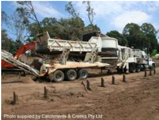
Tub-grinder mulch production
