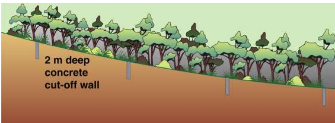
Concrete cut-off trenches
